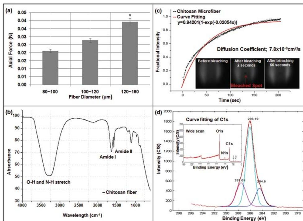
**Fig. 4** (a) Axial forces of synthesized chitosan fibers of three diameters ( $n = 3$ , \* indicates  $P < 0.05$ ). (b) ATR-FTIR surface analysis of a synthesized chitosan fiber. (c) FRAP data for diffusion of 70 kDa FITC-dextran in chitosan fibers; the fluorescence was fully recovered after photobleaching. (d) ESCA wide scan and C1s narrow scan with the curve fitting of chitosan.
