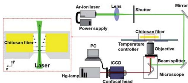
Fig. 2 FRAP system for measurement of diffusion in chitosan fiber.
