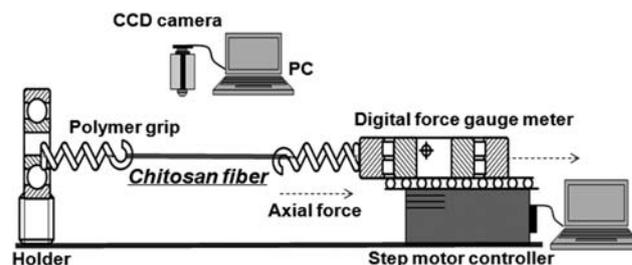
Fig. 1 Schematic diagram of axial force measurement system.
