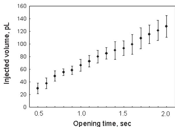
**Fig. 2** Graph showing the volume of the ejected solutions as a function of valve opening time. The volume of the ejected solution ranged from 30 pL to 130 pL and increased linearly with the length of opening duration.
