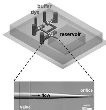
**Fig. 1** Schematic design of the Microfluidic Multi-Injector (MMI). Control channel and fluidic channel crossings make up the on-chip barrier valves (V1, V2, V3). These valves were actuated by pressurizing the control channel and deforming the membrane between the channels to close the fluidic channel. These valves controlled the pulsatile release of solution into the reservoir to generate a gradient. The micrograph shows the region around the barrier valve and the microfluidic orifice.
