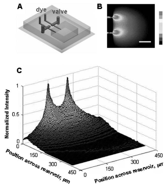
**Fig. 4** Generation of overlapping gradients in the MMI. (A) Schematic design of the parallel MMI on a single chip. Two parallel micro-injectors,  $120 \mu\text{m}$  apart, were simultaneously controlled by valves actuated at 0.67 Hz with 1 s opening. (B) 2D intensity profile of the fluorescence image showing symmetric overlapping gradients of FITC-Dextran. (C) 3D normalized fluorescence intensity profile. Scale bar represents  $100 \mu\text{m}$ .
