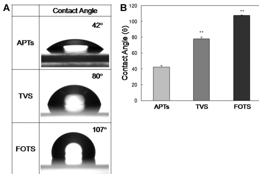
**Figure 2.** Contact angle measurements to determine hydrophilic and hydrophobic properties of materials. Contact angle images (A) and analysis (B) of APTs, TVS, and FOTS surfaces, indicating that the contact angles were 42°, 80°, and 107°, respectively. The contact angles of TVS and FOTS surfaces were compared with the APTs surface (\*\* $P < 0.01$ ).
