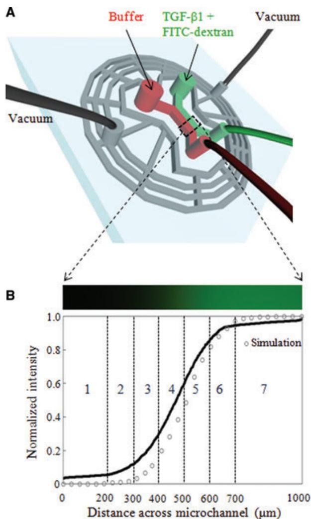
**Figure 1.** The microfluidic gradient device. (A) Schematic diagram of the microfluidic gradient device containing fluidic and vacuum network microchannels. (B) Experimental analysis and numerical simulation of the concentration gradient profiles in the microfluidic gradient device.
