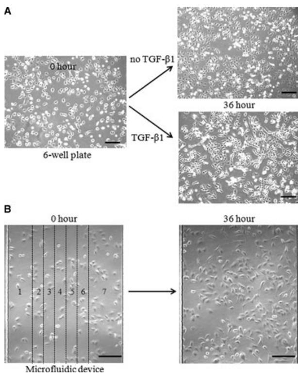
**Figure 2.** The growth of A549 human lung alveolar epithelial cells cultured in a 6-well plate and the microfluidic device. Phase contrast images of A549 cells that were cultured with or without TGF- $\beta$ 1 in a 6-well plate (A) and the microfluidic gradient device (B). Scale bars are 200  $\mu$ m.
