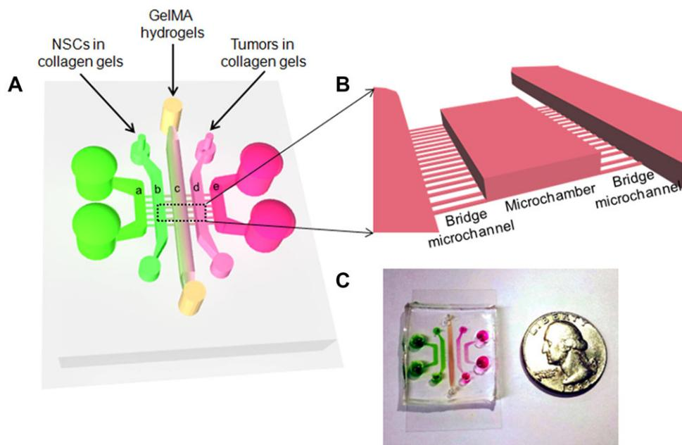
**Figure 1.** Photo-crosslinkable hydrogel-based 3D microfluidic culture device. (A) Schematic drawing of the photo-crosslinkable hydrogel-based 3D microfluidic device containing five microchambers and four bridge microchannels. (B) Schematic of cross-sectional the photo-crosslinkable hydrogel-based 3D microfluidic culture device. (C) Photograph of photo-crosslinkable hydrogel-based 3D microfluidic culture device.
