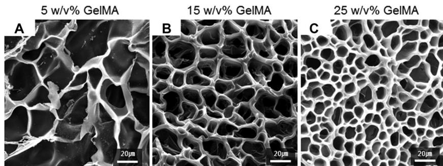
**Figure 2.** SEM images of (A) 5 w/v%, (B) 15 w/v%, and (C) 25 w/v% photo-crosslinkable GelMA hydrogels. Scale bars are 20  $\mu\text{m}$ .
