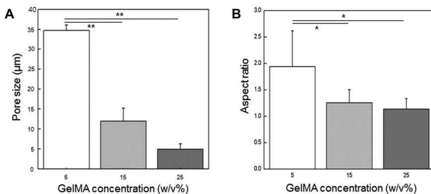
**Figure 3.** Effect of GelMA hydrogel concentrations (5–25 w/v%) on (A) pore size and (B) aspect ratio. The aspect ratio means the ratio of the length of pores divided by width of pores ( $*p < 0.05$ ,  $**p < 0.01$ ).
