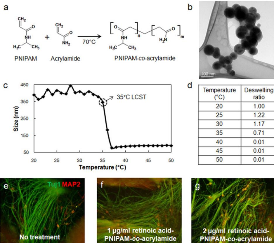
**Fig. 3.** PNIPAM nanocomposite-mediated human iPSC differentiation. (a) Polymeric nanocomposites containing PNIPAM and acrylamide. (b) TEM image of PNIPAM-co-acrylamide nanocomposites. (c-d) Size distribution and deswelling ratio of PNIPAM-co-acrylamide nanocomposites. (e-g) Human iPSC-derived neuronal differentiation using retinoic acid-loaded PNIPAM-co-acrylamide nanocomposites. (reprinted with permission from ref. 34, copyright 2015 Elsevier).
