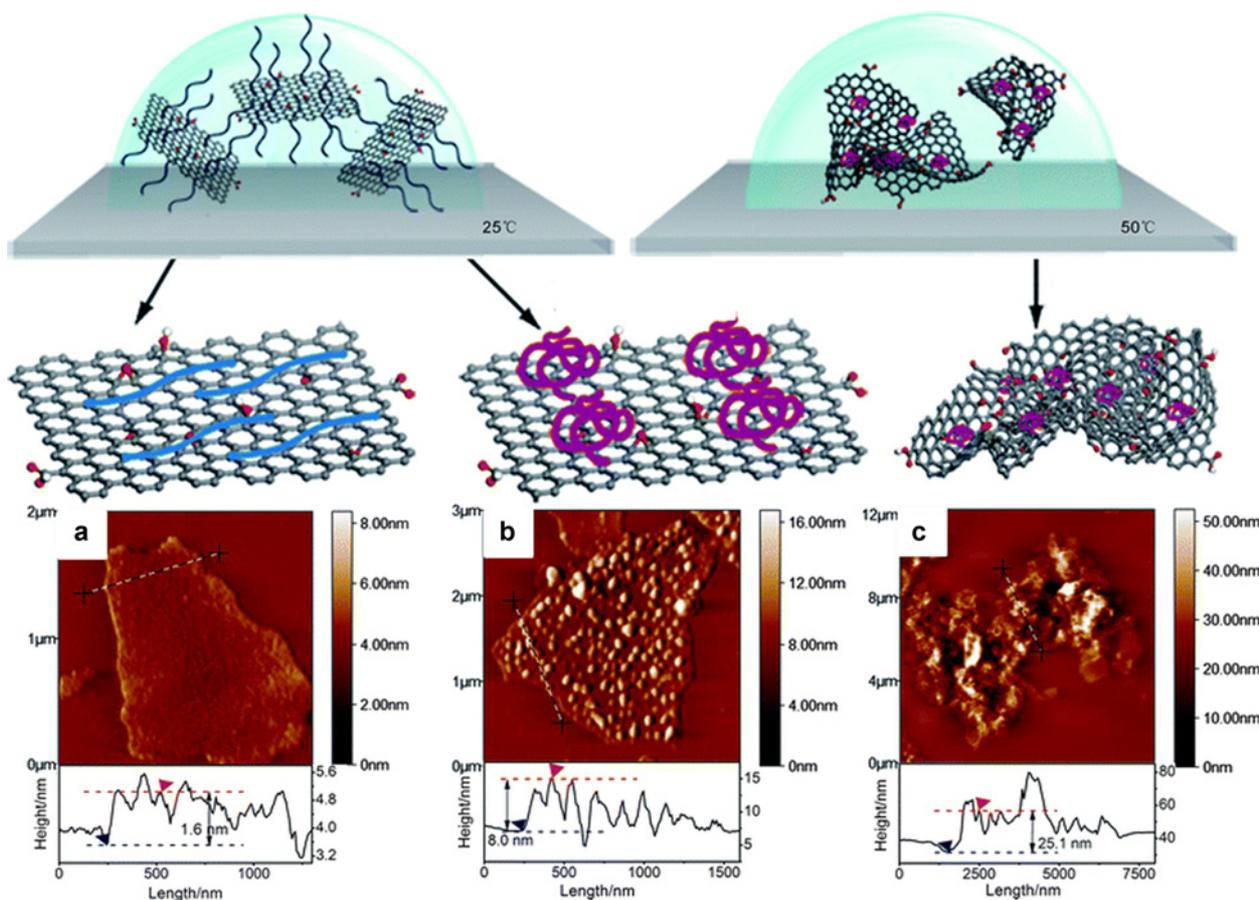
**Fig. 1.** AFM image analysis of a droplet of graphene oxide-based PNIPAM nanocomposite suspension at different conditions: (a) fully dried at 25°C, (b) partially dried at 25°C and heated at 50°C, and (c) heated and fully dried at 50°C. (reprinted with permission from ref. 23, copyright 2012 Royal Society of Chemistry).
